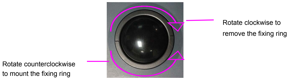
Figure 13-1 Assembling and Disassembling Trackball
